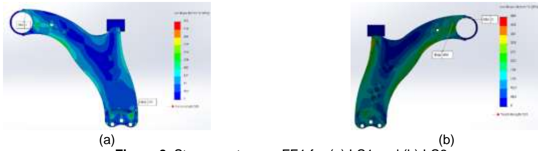
Figure 2. Stress contour on FE1 for (a) LC1 and (b) LC2.
