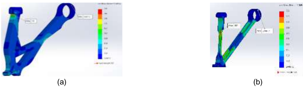
Figure 4. Stress contour for LC2 of (a) FE3 and (b) FE4.
